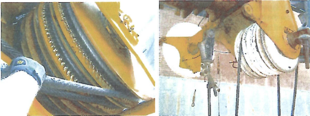
Fig. 3 Usual steel sheaves, left, hard & heavy; Synthetic sheaves, right, lighter and easier on the rope
