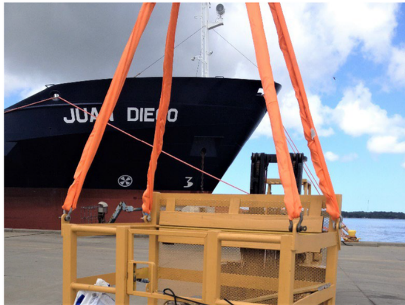
Fig. 2 Synthetic "round slings," Low cost, handleability, and lightweight – just user-friendly!
